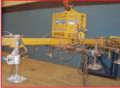
ANVER Vacuum Sheet Lifter, 1,000 lb Capacity, sn 51000189
