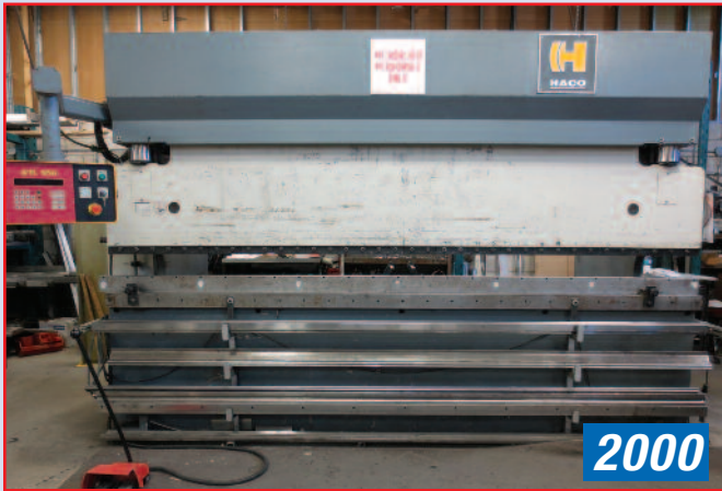
HACO 165 Ton x 12' Press Brake, Model PPM-36-150, ATL 550 3 Axis CNC Back Gauge, Distance Between Uprights 124", Microguard Light Curtains, 575V, sn 90484
