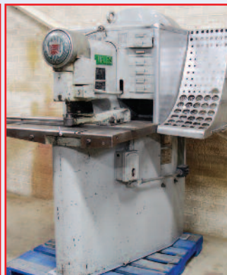
WALES STRIPPIT 25 Ton Punch, 15" Throat, 23"x30" Table, 20" Arm Extension, Large Selection Assorted Punches & Dies, sn 31632859
