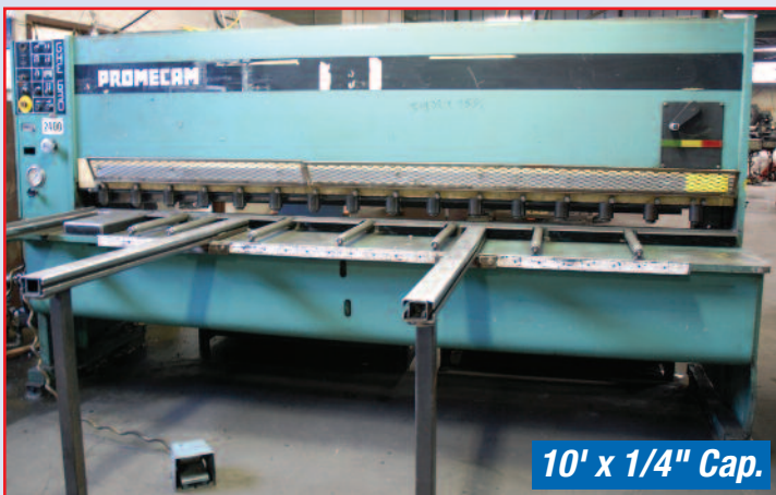
PROMECAM Hydraulic Shear Model GHE 630, Squaring Arm, Support Arms, Front Operated Power Backgauge, sn 213
