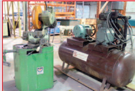
BEWO Cold Saw + 5 HP Compressor
