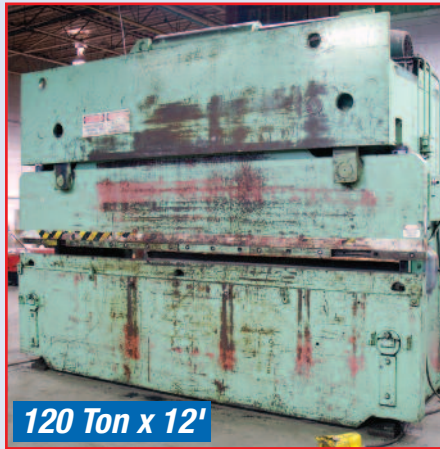
ALLSTEEL Press Brake, Distance Between Frames 10'6", Variable Stroke 0-8", Open Height 17", 15 HP, sn 2075
