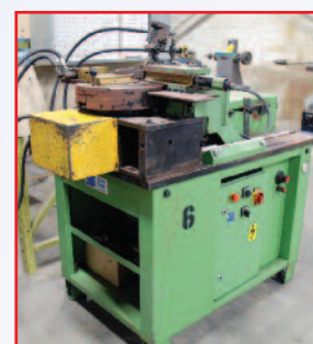
1999 STIERLI-BIEGER 2", 33 Ton Hydraulic Tube Bender, Model 300HE / CEB9, Adjustable Stroke up to 11-3/8", 7.5 HP, sn 151 Custom Pipe Bender
