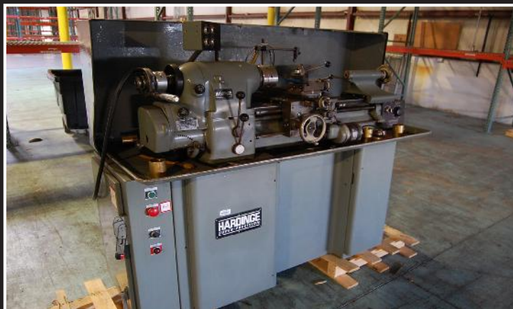
Hardinge Super Precision engine lathe; 1 1/4" hole through center, 10" swing, 18" center to center, carriage feed
