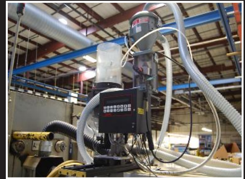
Van Dorn 120-HT-8F injection molder; 1994 vintage, RS rotating screw, clamp tonnage 230 max, 20 ounce injection unit capacity, serial 547
