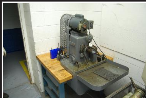
Sunnen MBB625D precision honing machine; spindle speed 300 -800 rpm's, serial 13674
