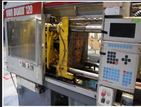
Van Dorn 120-HT-8F injection molder; 1994 vintage, RS rotating screw, clamp tonnage 230 max, 20 ounce injection unit capacity, serial 547
