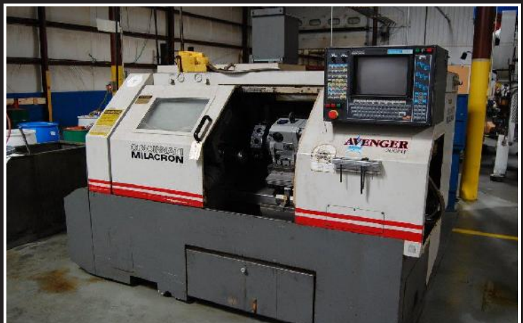
Cincinnati Milacron Avenger 200 MT CNC turning center; 12 position tool holder, Acramatic 850 SX controls, serial 3650AMT96-0009
