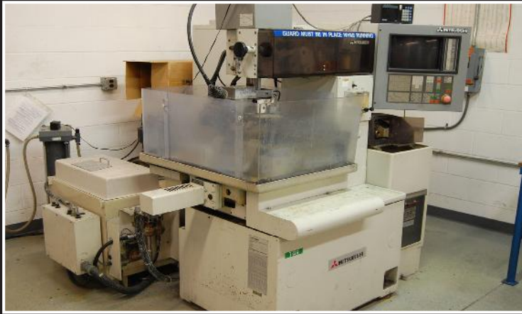
Mitsubishi DWC90CR wire EDM machine; 1996 vintage, Sony X readout, serial 069D1422
