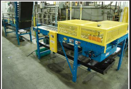
Bastian Automation Engineering conveyor system consisting of: (1) 12" capacity Hytrol powered conveyor, (1) 10' section, (1) 7' section with 20" capacity, (1) 45' section with 20" capacity
