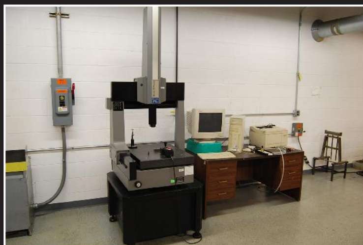
Brown & Sharpe Micro Val PFX coordinate measuring machine; 22" x 29 1/2" granite surface table, serial 112218
