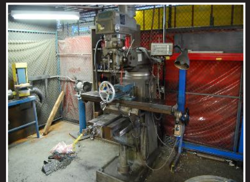
Nantong vertical milling machine; 10" x 54" table, spindle speed 70 - 600 rpm's, Mitituyo x/y readout, left to right power feed, serial 41586
