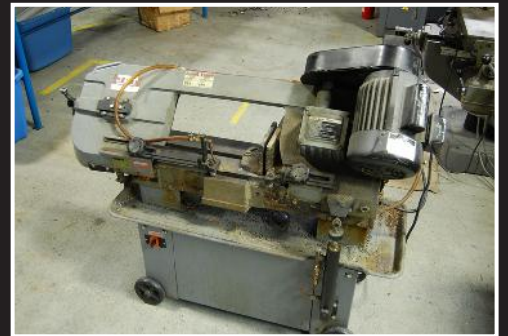
Jet HUBS 7MW horizontal/ vertical band saw; 3/4 hp, single phase, 1994 vintage, serial 414459
