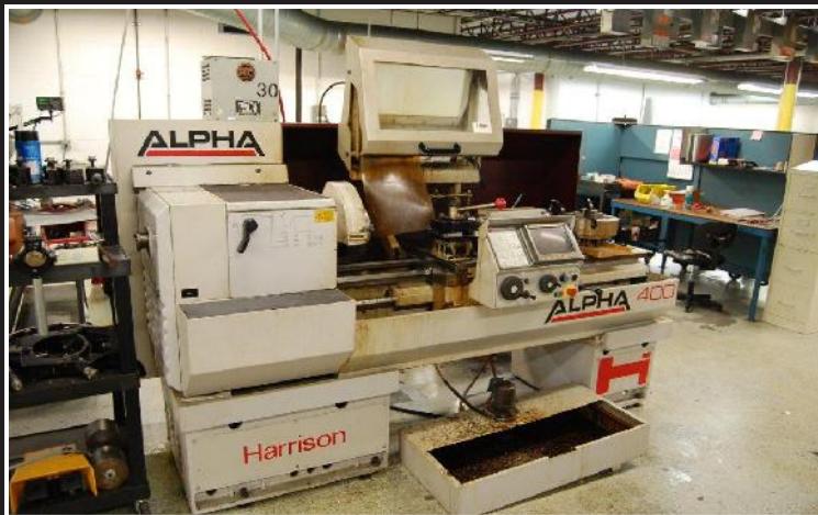
Harrison Alpha 400 engine lathe, spindle speed 15 - 2500 rpm's, 16" swing, 1 1/4" hole through center, 44" center to center, GE Fanuc x/z control, serial A30531-0400
