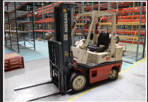
Nissan KCPH02A25PV Enduro 50 fork lift; 4400 lb lift capacity, 187" lift height, 3 stage mast, side shift, 42" forks, 4957 hours on meter, L.P. powered, serial KCPH02P908761
