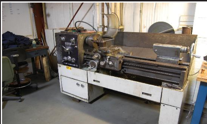
Southbend Nordic 15 engine lathe; spindle speed 40 - 2000 rpm's, 2" hole through spindle, 8" swing, 30" center to center, 57" bed, serial CN700228B79
