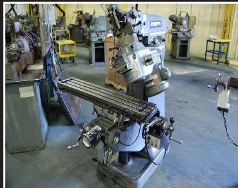
Bridgeport vertical milling machine; spindle speed 500 - 4200 rpm's, 9" x 48" table, Bridgeport 8F power feed, serial 266312
