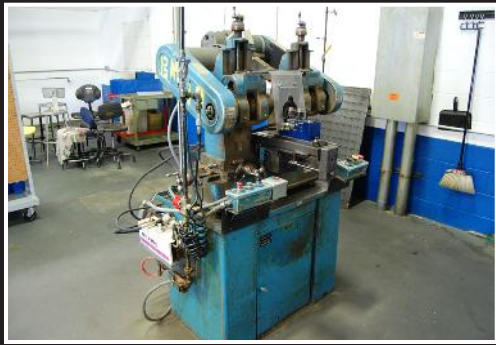
Barker model AMP milling machine; spindle speed 350 3060 rpm's, coolant, SPX Hytec hydraulics for Hardinge 5C collet holder, serial 1505B
