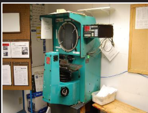
J & L Tec 14 optical comparator; 14" screen, Quadra Check 2000 digital readout, 5" x 20" table
