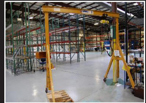
Spanco 1 ton "A" frame portable gantry; 114" wide with adjustable height, Budgit 250 lb electric hoist
