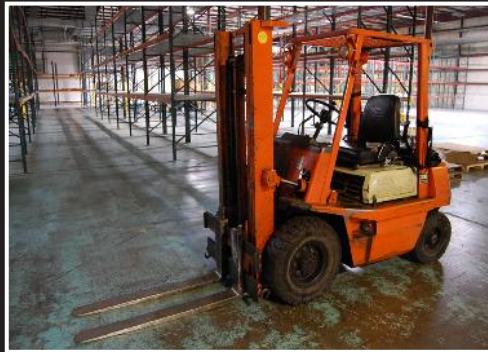
Toyota 3FGL20 fork lift; 3000 lb lift capacity, 2 stage mast, 48" forks, 120" lift height, L.P. powered, serial 3FGL25-12813
