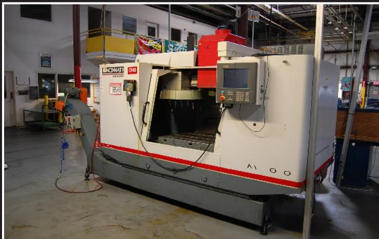
Cincinnati ERM Arro 1000 CNC milling machine; 20 position tool holder, chip conveyor, 24" x 44" table, Cincinnati Acramatic A2100 controls, coolant, serial 7049-A00-99-0769
