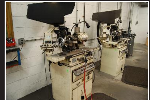
Royal Oak form relief grinder; 12" optical comparator attachment, Accurite X/Y read-out, Universal Form relieving fixture, serial 25R0244
