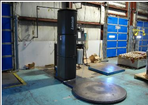
Lantech Q300 stretch wrapper; 115/20, 60" table, serial Q2075
