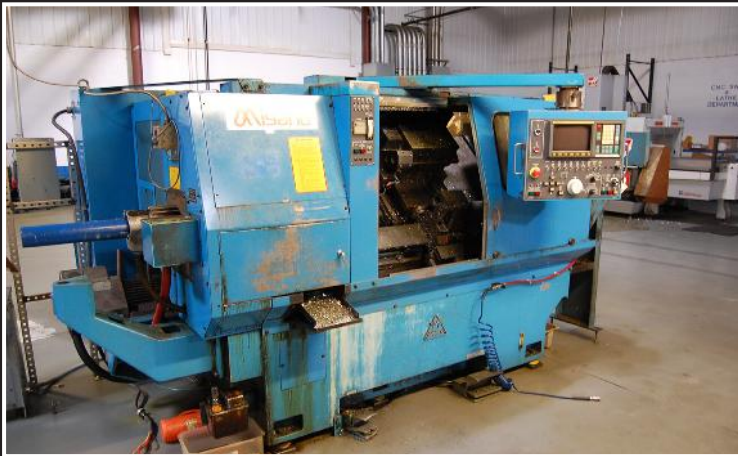
Miyano JNC 45 CNC machining center; Fanuc OT controls, chip conveyor, coolant, 8 position tool holder, serial JN450553
