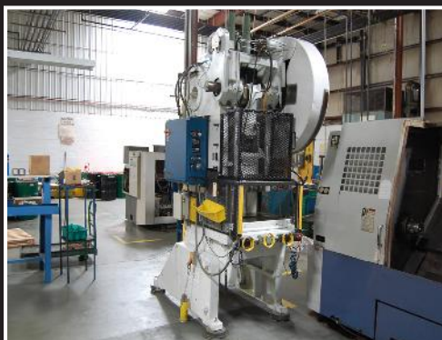
Bliss C60 OBI punch press; slide adjust 3, shut height 14 1/4", Cienco PC1-100 controls, Micro Safe light curtains, air counter balance, 4" shut height, serial H61646HP47139
