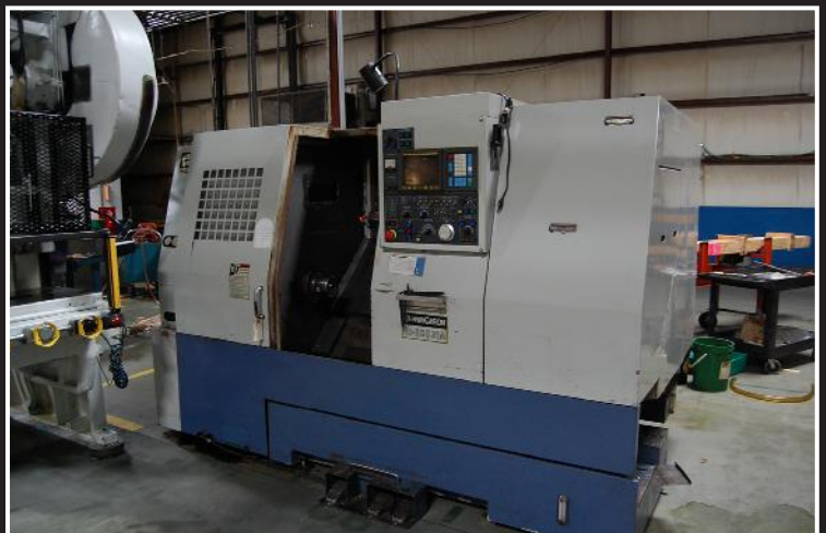
Hwa Cheon H1 ECO 31A CNC turning center; 1994 vintage, IO Position tool holder, Fanuc Korea O-T series controls, serial 94051753
