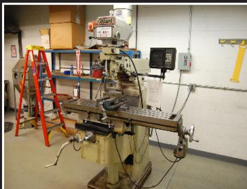
Alliant 1054-V3 vertical milling machine; spindle speed 70 - 4200 rpm's, Anilam Wizard 150 Plus X/Y readout, 10" x 54" table, left to right power feed, serial K3VL-1143
