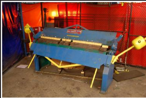
Jet SBR30N shear/ brake/ roll combo; 20 gauge x 30" capacity, stock 754031
