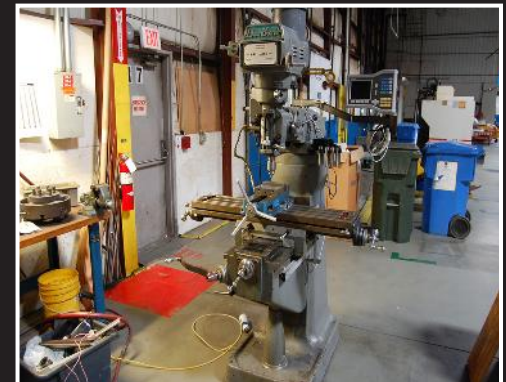
Hartford M05-10MD vertical milling machine; 9" x 42" table, spindle speed 60 - 4200 rpm's, Accurite digital read out, serial 8812050
