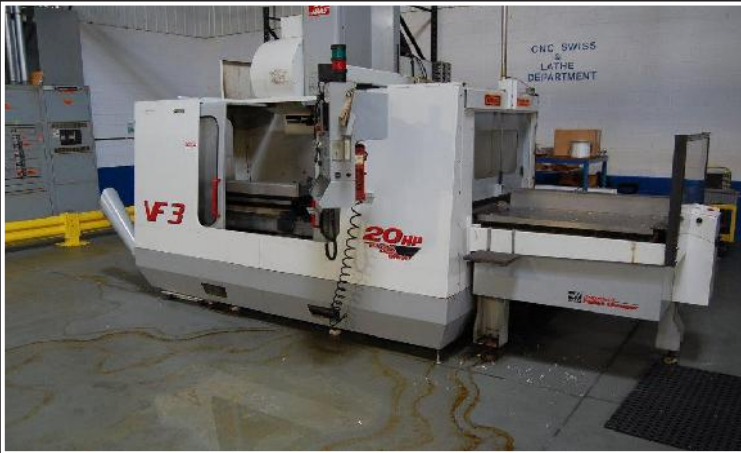
Haas VF3 CNC machining center; 2000 vintage, 24 position tool holder, 19" x 40" table, automatic pallet changer, 20 h.p. Vector Dual drive, Haas programmable coolant, serial 21536
