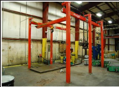
Snap Trac 1/2 ton hoist; freestanding 150" span x 16' run, hook to floor 8'
