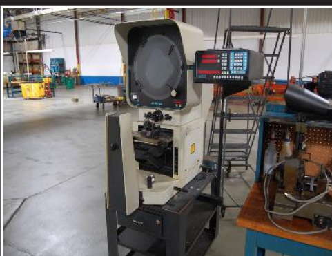
Deltronic DH 124 optical comparator; 14" screen, 5" x 15" table, Gage Master x/y readout, serial 249083754
