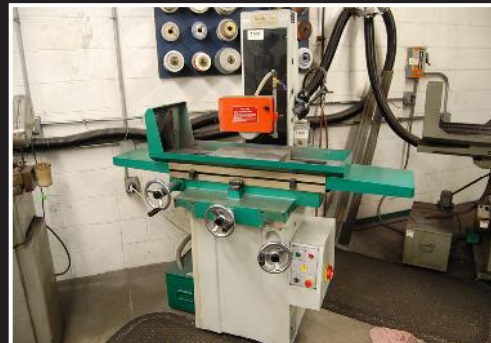
Grizzly model G3155 surface grinder; 2 hp, spindle speed 3450 rpm's, 16" x 8" table, manual magnetic chuck, 2006 vintage, serial 06051354
