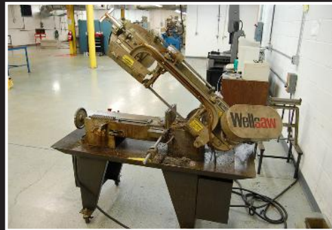
Wellsaw 613 horizontal band saw; .75 X .032 x 98.5 blade size, 13" window, serial 1414
