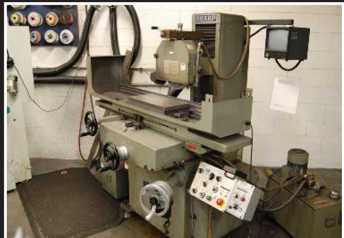
Sharp model SH920 hydraulic surface grinder; 10" x 19 1/2" electro magnetic chuck, 1999 vintage, serial 90905-04
