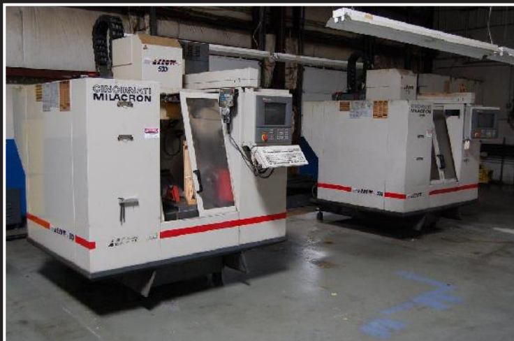
Cincinnati Milacron ERO Arro 500 CNC milling machine; 21 position tool holder, 20 1/2" x 27 1/2" table, Vickers Acramatic 2100 controls, coolant, serial 7042 A00 96 0859
