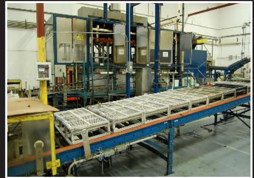
FRI Systems finshing and cleaning system; (2) stage washing, (2) stage rinsing, (1) stage drying, powered conveyor with 40" x 20" baskets
