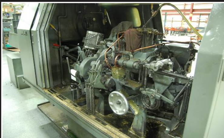
(10) Davenport HP 5 spindle CNC screw machines; Noise Tamer, spindle pick off and deburring, bar capacities = round @ 0.875", hex @ 0.750" and square @ 0.625"
