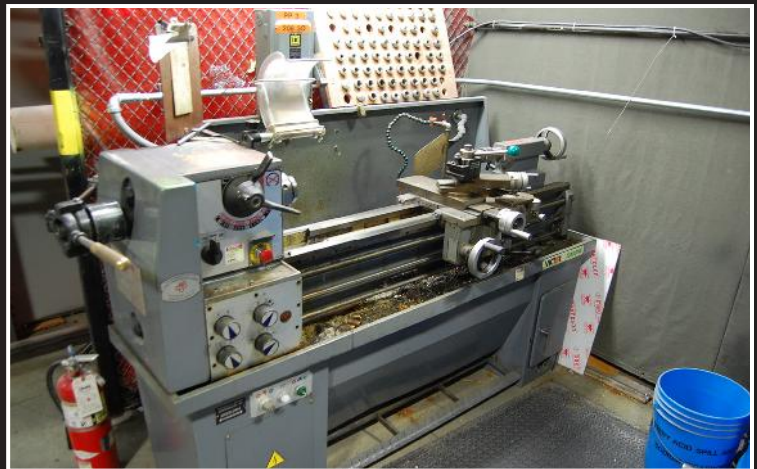
Victor 1340 GHE engine lathe; 6 3/4" swing, 30 1/2" center to center, 53" bed, 1 1/4" hole through spindle, spindle speed 70 - 2000 rpm's, serial 18303023
