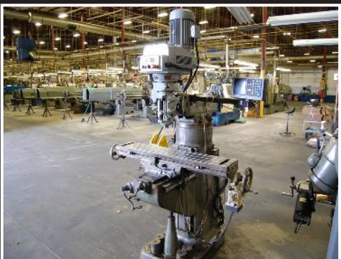
Bridgeport model 137992 vertical milling machine; Acer head, spindle speed 60 - 4500 rpm's, 9" x 48" table, left to right power feed, Accurite X/Y digital readout, serial 137992
