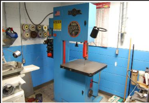
Do All 2013-V band saw; 12' x 10" blade, with welder & grinder, 26" x 26" table, 20" throat, 13" max height, serial 500-95834
