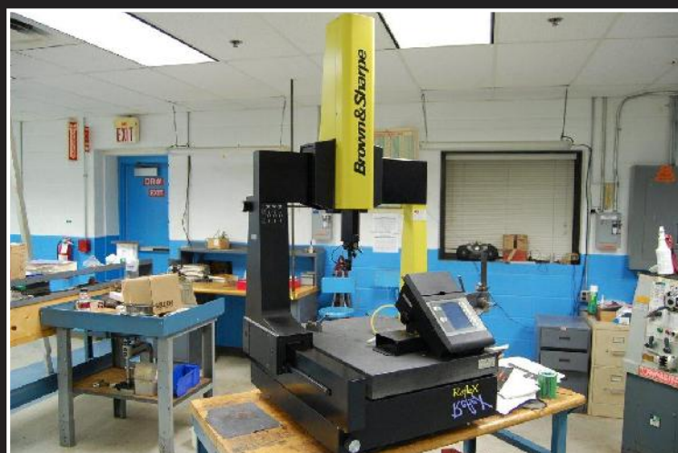
Brown & Sharpe Reflex coordinate measuring machine, 500 lb max, 29 1/2" x 22" granite surface table, serial 0197-1513
