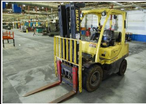
Hyster H60 Fortis fork lift; 5700 lb capacity, L.P. powered, 3 stage mast, 170" lift height, side shift, 42" forks, 2638 hours, serial L177B23754F
