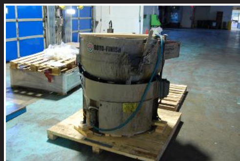
Roto Finish 3608 tumble finisher; 40" diameter, Spiratron Extended Range series, serial ER-0203S-95-C14
