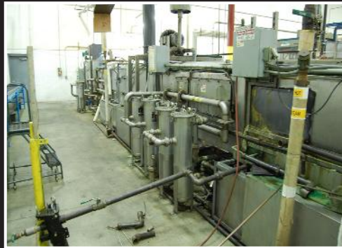
CDF parts washing machine; 23" x 8 1/2" opening, approximate 50' length, includes (6) Rosedale filtration units
