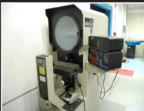
Micro Vu M103 optical comparator; 14" screen diameter, Micro Vu x/y/z readout, 5" x 18" table, serial 5901
