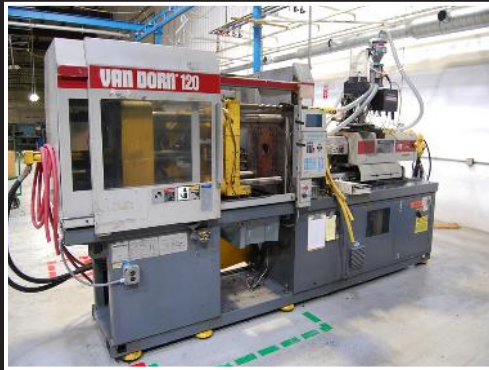
Van Dorn 120-HT-8F injection molder; 1994 vintage, RS rotating screw, clamp tonnage 230 max, 20 ounce injection unit capacity, serial 547
