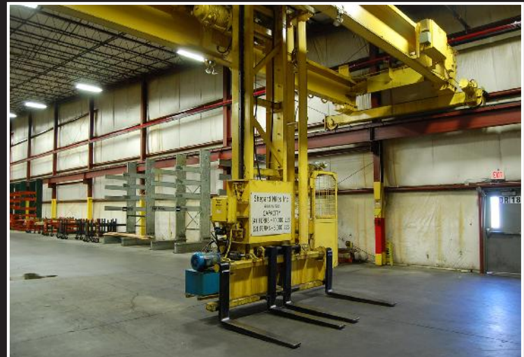
Shepard Niles Inc. fork lift style overhead rotating lifting/ transport system; (4) forks rated at 10,000 lbs, (2) forks rated at 5,000 lbs, approximate 37' span, approximate 368' runway, width between outer forks = 115" and interior forks = 38", serial 72165
