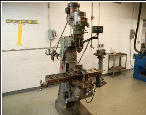
Bridgeport Series 1 vertical milling machine; 2 hp, spindle speed 500 - 4200 rpm's, Sony X/Y readout, left to right power feed, 9" x 42" table, serial 185293
