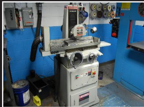
Harig (by Bridgeport) Ballway hydraulic surface grinder; 6" x 18" manual magnetic chuck
