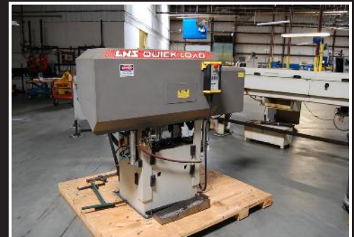
LNS Quickload bar feed; 1997 vintage, serial 24278
