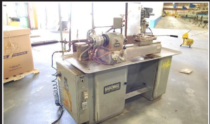
Hardinge model DSM-59 super precision engine lathe; 1 hp, 8" swing, 18" center to center, 1 1/4" hole through center, Gusher coolant system
