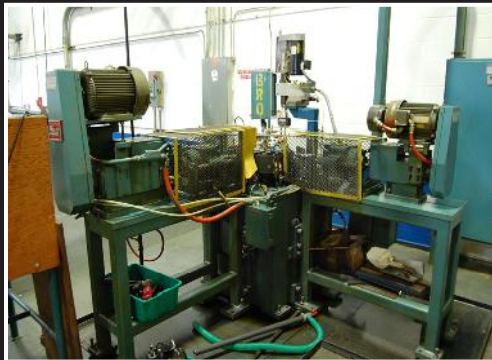
Drilling & Tapping machine; custom made, consists of Ettco model 500 and model 4 drills, ARO model 47276 twin spindle with rotary table
