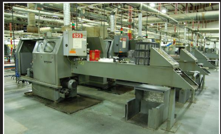
(10) Davenport HP 5 spindle CNC screw machines; Noise Tamer, spindle pick off and deburring, bar capacities = round @ 0.875", hex @ 0.750" and square @ 0.625"
