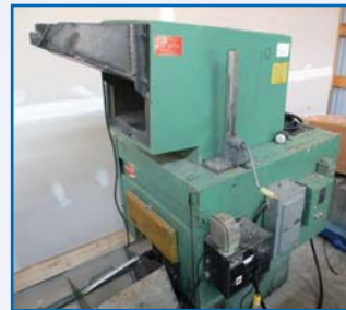
1993 CINCINATTI MILACRON 6065 AUTOBLOW single extrusion, single die blow molder with single die-head with machine trim, visi-stripe capable, vacuum loader, 480 volt s/n na #10
