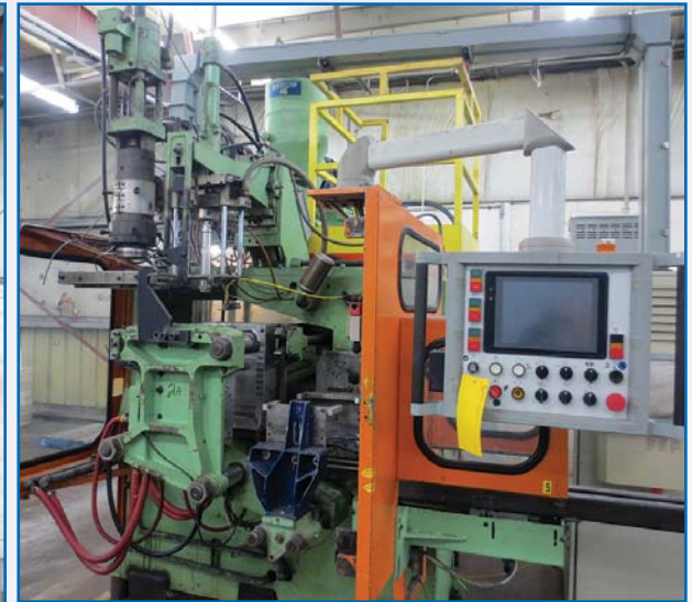
1991 BEKUM H-155 single extrusion, double die blow molder with MACO 8000 control, 90mm extruder, 11.2 ton clamping force, 2 sec. dry cycle, molds: 480mm width, 470mm length, (2) 130mm depth, 220mm daylight, vacuum loader, 480 volt, comes with (2) 5L F-Style Jug molds, 38-400 neck size s/n 155D004.5 #12
