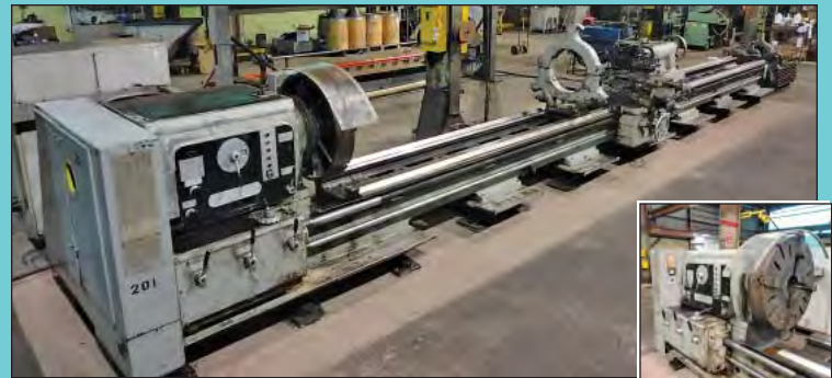
Reverse View 40" / 52" X 320" Poreba Model TR-100B1/8M Geared Head Gap Bed Engine Lathe
