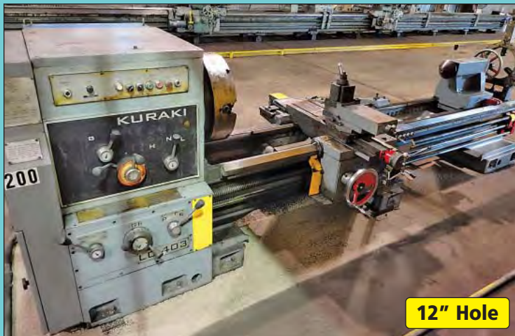
Reverse View 32" X 120" Kuraki Model LC-403-30 Hollow Spindle Geared Head Engine Lathe
