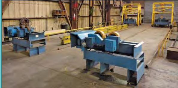
(2) 50' Long Mfg. Unk. Custom Built Traveling Gantry Manual Shaft Straightening Systems
