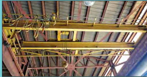
(3) 7 -1/2 Ton X 26' Approx. Span Pelham Double Girder Top Running Overhead Bridge Cranes; (2) w/Remote Controls
