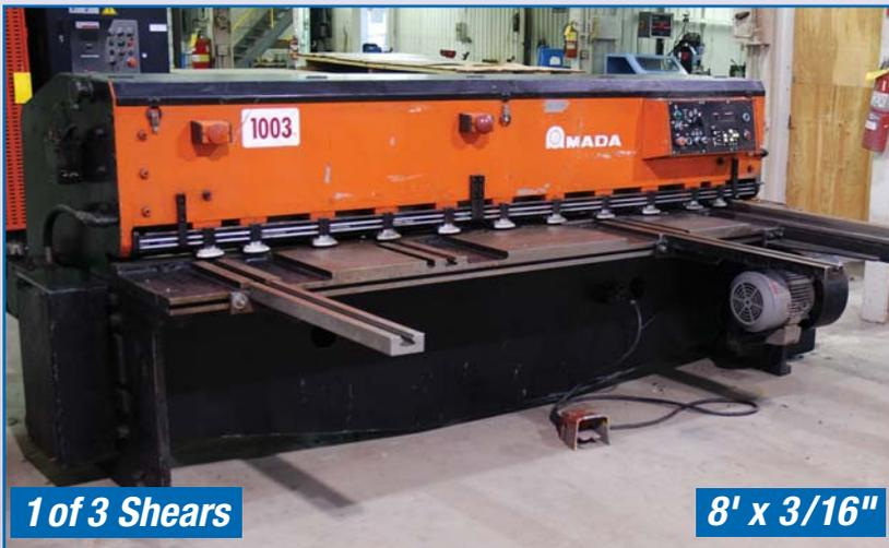
AMADA MODEL M2545 MECHANICAL SHEAR
