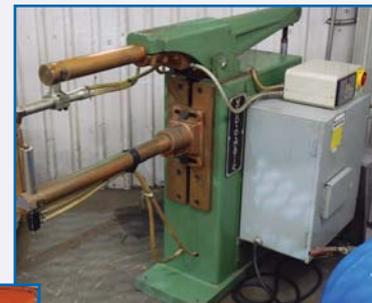
**WELDOMATIC** 50 KVA SPOT WELDER, MODEL AF-2B
