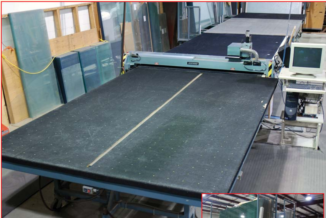
LOCKFORMER MODEL EXCALIBUR E612F DIAMOND TIP CNC OPTIMIZING GLASS CUTTER WITH GF TECHNOLOGIES BREAK OUT & FLOAT TABLES
