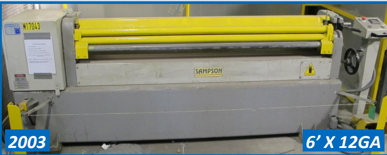
SAMPSON-AKAYPAK MODEL MRM-640 PLATE BENDING ROLL
