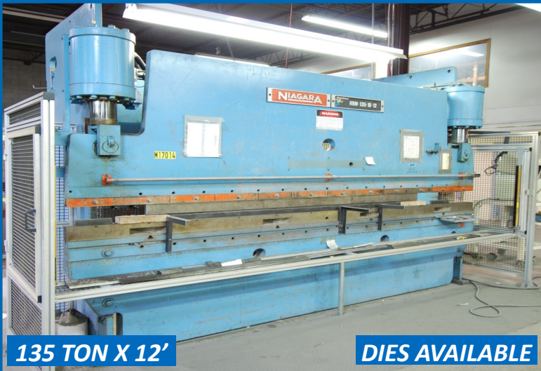
NIAGARA MODEL HBM-135-10-12 HYDRAULIC CNC PRESS BRAKE
