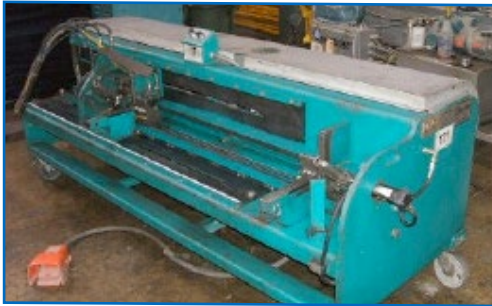
IOWA MODEL FAH-1872-HP SEAM CLOSER
