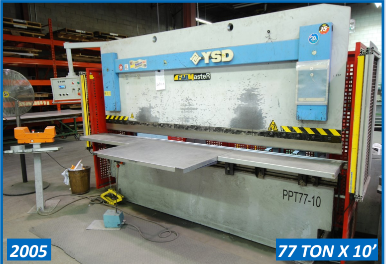
FABMASTER YSD MODEL PPT-77-10 HYDRAULIC PRESS BRAKE
