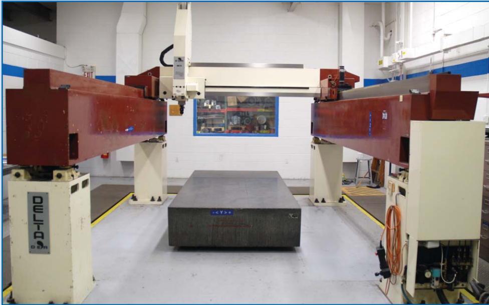
DEA Delta 3406 DCC CMM, Travels: X-72", Y-120", Z-54", Granite Table Size 60"x120"x18", Renishaw PH10M Probe, sn 3406
