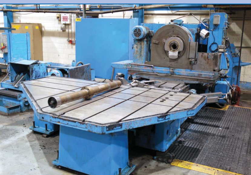
LUCAS Model 42B-60, Table Size 86"x48", Travels: X-74", Y-36", Z-84", Spindle Dia 5", CTS, Drawbar, 10-1,220 RPM, 25 HP, 460V, sn 42B4234 [9]
