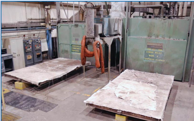
(2) LINDBERG Car Bottom Furnaces (Stress Relief, Bake, Tempering, Age etc.) 8' W x 14'L x 5'H, Working Range 375-575 F
