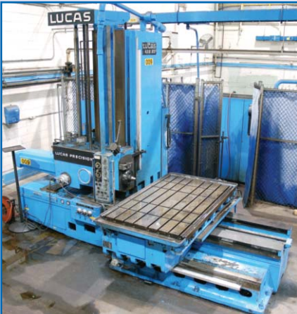
LUCAS Model 42B-60, Table Size 86"x48", Travels: X-74", Y-36", Z-84", Spindle Dia 5", CTS, Drawbar, 10-1,220 RPM, 25 HP, 460V, sn 42B4234 [9]
