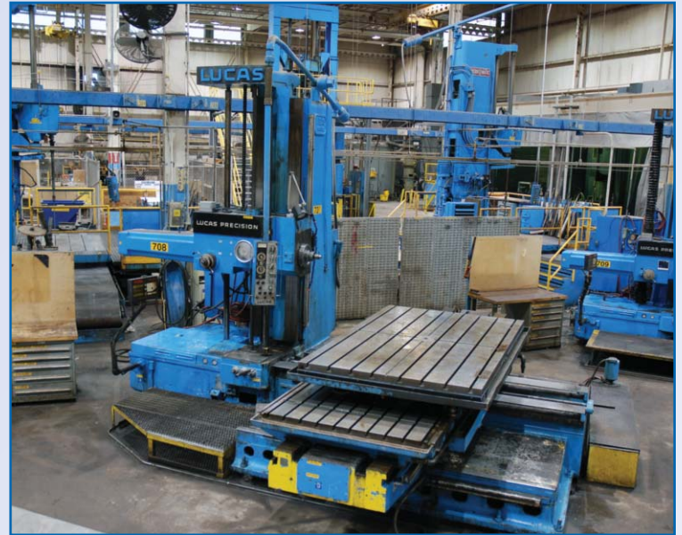
LUCAS Model 542B120, Travels: X-108", Y-60", Z-84", Table Size 56"x122", Additional Rotary Table Size 60"x96", 5" Spindle Dia, Cat 50, Max 1,220 RPM, CTS, Drawbar, Renishaw Probe, 35 HP, 460V, sn 42B4208 [708]
