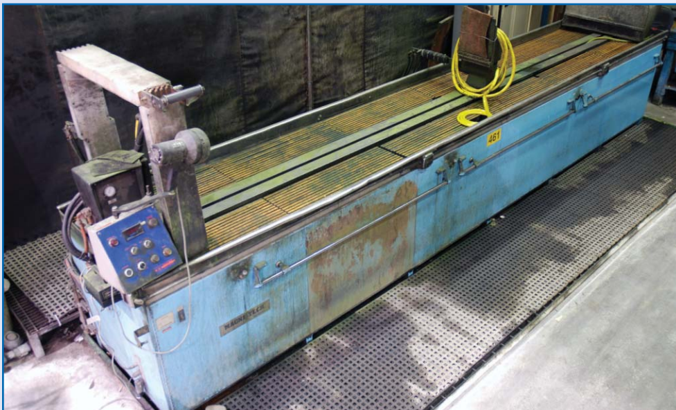
MAGNE-TECH Gould Bass Magnetic Particle Inspection Unit, Model 3509C-10S, 19' x 38" Bed, Dual 13"x13" Clamp Contacts, Test Bars, sn 083003 [461]
