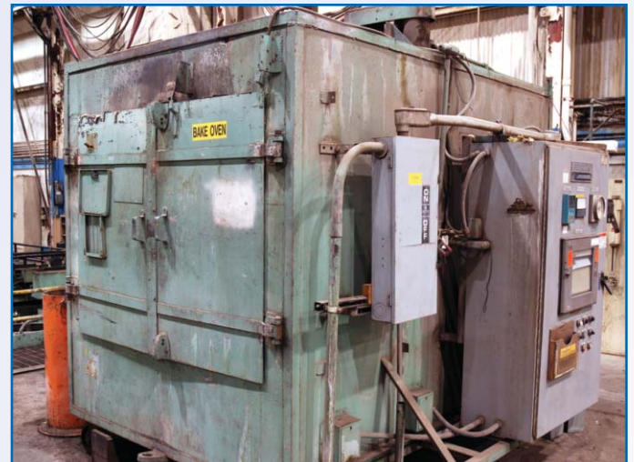
LINDBERG Bake Oven, Digital Controller, Temp Chart, Interior Dimension 66"x96"x58", Class IV Type D, TUS Tolerance +/- 25F, Working Range 375-525 F, Temp 250 Deg, Gas Volume 6000 CFH, 440V [403]
