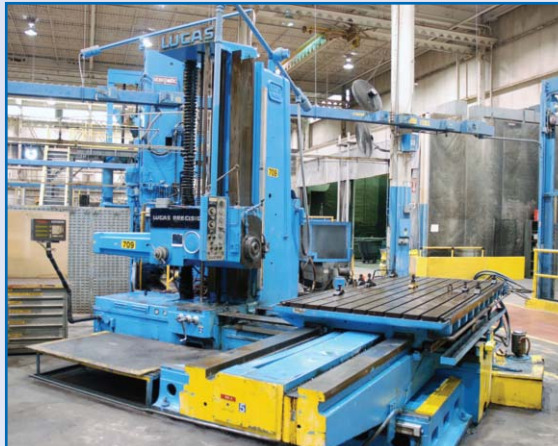
LUCAS Model 542B120, Travels: X-108", Y-36", Z-84", Table Size 56"x122", 5" Spindle Dia, Cat 50, Max 1,220 RPM, CTS, Drawbar, Renishaw Probe, 35 HP, 460V, sn 42B4126 [709]
