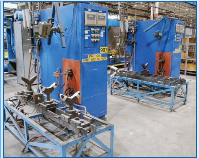
(2) AJAX MAGNATHERMIC Induction Heaters, For Stress Relieving and Homogenizing of Large Welded Parts, 7"x2.5" Heated Platen, 31"x79" Work Tables, Pacer S10 Control, sn HK-2B400-ABD-1 & ABD-2 [906, 907]
