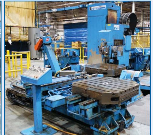
KEARNEY & TRECKER 5 Axis Machining Center, Model Modu-Line, System Gemini Control, Dual 40"x40" Pallets, 50 Taper, 39 ATC, Chip Conveyor, sn 4885121 [196]
