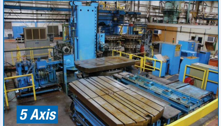
(2) KEARNEY & TRECKER 5 Axis Machining Centers, Model Maxi-Bar, Gemini D17 Control, Dual 10'x6' Rotary Shuttle Tables, Travels: X-133", Y-96", Z-48", 6" Spindle, Cat 60, 144 ATC, U-Axis Capability, D'Andrea Facing Head, 20" Max Dia., Full 5 Axis Contouring, Spindle Speed Range 8-1,570 RPM, CTS, Drawbar, Renishaw MP-9 Probe, Chip Conveyor, DC Axis Drive Servos, 50 HP, 480V, sn's 8787267 & 8784254 [197 & 199]
