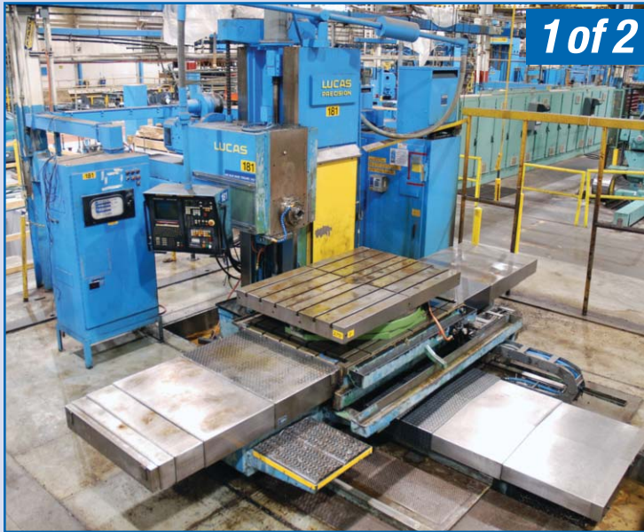
(2) LUCAS CNC Horizontal Boring Mills, Model 30T65, GE Mark Century 2000 Control, Table Size 4'x6', 4'x6' Rotary Table, Travels: X-72", Y-60", Z-36", W-48", CTS, 460V, sn's 30T1302 & 30T1303 [180 & 181]
