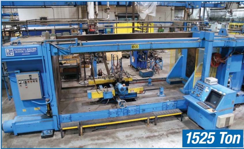
AMD Pressure Welder, Model 1526-30, 1525 Ton, Control Electronics Model 6152, Center Height From Top Of Table 31", Fixed Platen 99.5"x79", Moving Platen 60"x55", Gap Between Upper Beams 70", Max Part Size 16" x 75", Fixture Carriage, Brooks Instrument DRO, [430]
