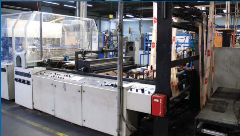
1996 LEMO MERCHANDISE BAG LINE, UTECO 6 COLOR PRESS, 63" WEB WIDTH, UP TO 250 BAGS/MIN (LINE 9)
