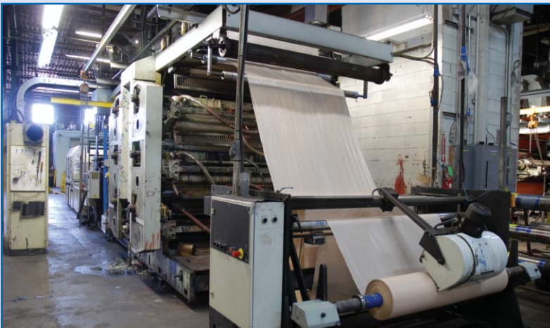
2002 SALDOFLEX T-SHIRT & MERCHANDISE BAG LINE WITH AUTOPACK, FILIPPINI & PAGANINI 6 COLOR PRESS 63" WEB WIDTH, UP TO 300 BAGS/MIN (LINE 1)
