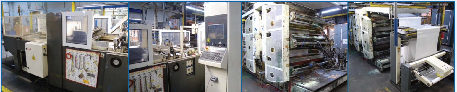
1999 SALDOFLEX T-SHIRT & MERCHANDISE BAG LINE, UTECO 6 COLOR PRESS, 63" WEB WIDTH, 250 BAGS/MIN (LINE 6)
