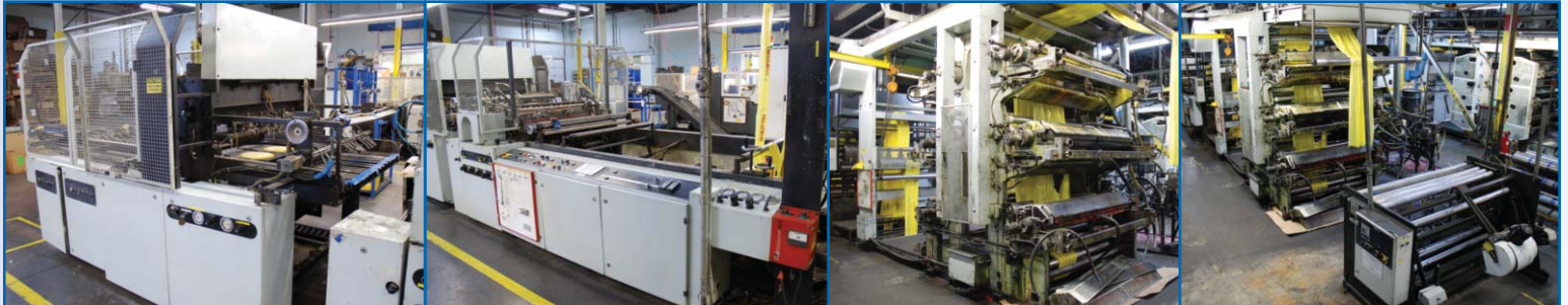
1996 LEMO T-SHIRT BAG LINE, UTECO 6 COLOR PRESS, 60" WEB WIDTH, 250 BAGS/MIN (LINE 7)
