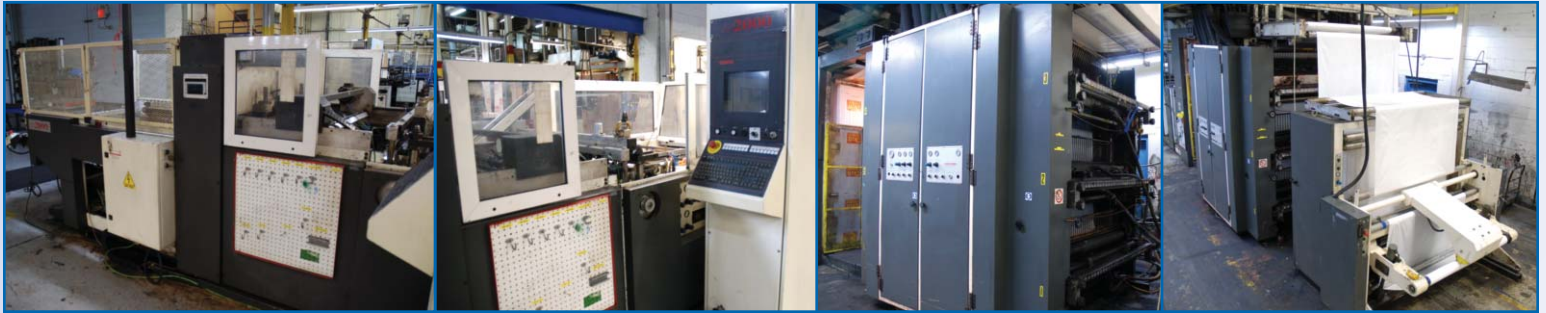
2000 SALDOFLEX T-SHIRT & MERCHANDISE BAG LINE, FILIPPINI & PAGANINI 6 COLOR PRESS, 63" WEB WIDTH, 275 BAGS/MIN (LINE 5)
