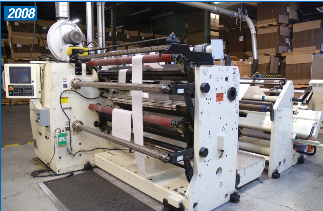
2008 DEACRO Slitter Model C610B-185, Duplex Cantilevered Re-Winder, Max Unwind OD 50", Unwind & Rewind Core Size 3", 48" Diameter, Max Unwind Roll Weight 5,000 lbs, Shaftless Floor Pickup Unwind, Max Web 70", Slit Width Range 1" – 70", Max Speed 1,500 FPM, Film Gauge Range 0.45 mil - 7 mil, Edge or Line Guide, Max Rewind Roll OD 24", Trim System, 10 HP Blower, Unloading Cart, sn 1596-562
