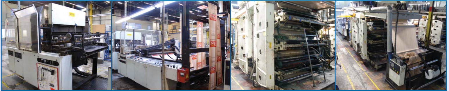
1996 LEMO T-SHIRT BAG LINE, UTECO 6 COLOR PRESS, 63" WEB WIDTH, 250 BAGS/MIN (LINE 4)
