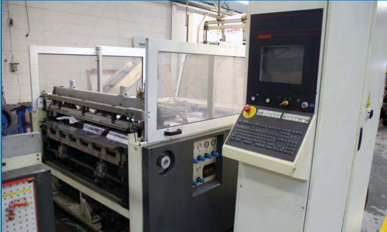
2002 SALDOFLEX T-SHIRT & MERCHANDISE BAG LINE WITH AUTOPACK, FILIPPINI & PAGANINI 6 COLOR PRESS 63" WEB WIDTH, UP TO 300 BAGS/MIN (LINE 1)
