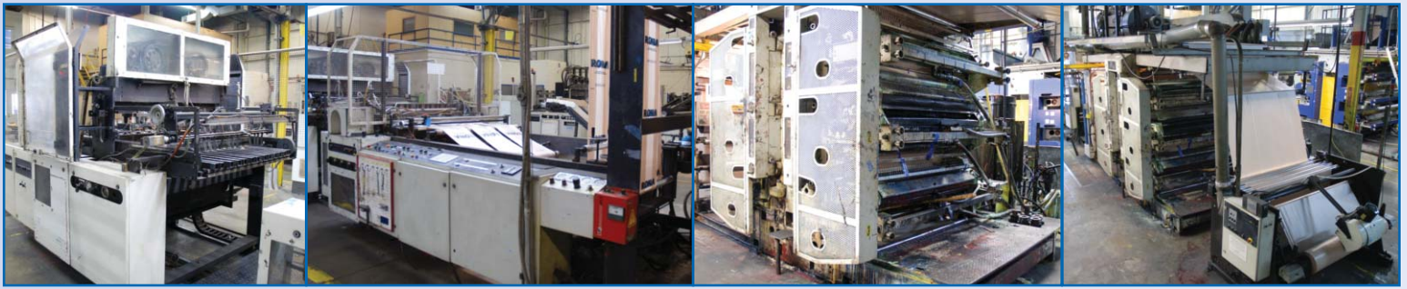
1996 LEMO T-SHIRT BAG LINE, UTECO 6 COLOR PRESS, 63" WEB WIDTH, 250 BAGS/MIN (LINE 3)
