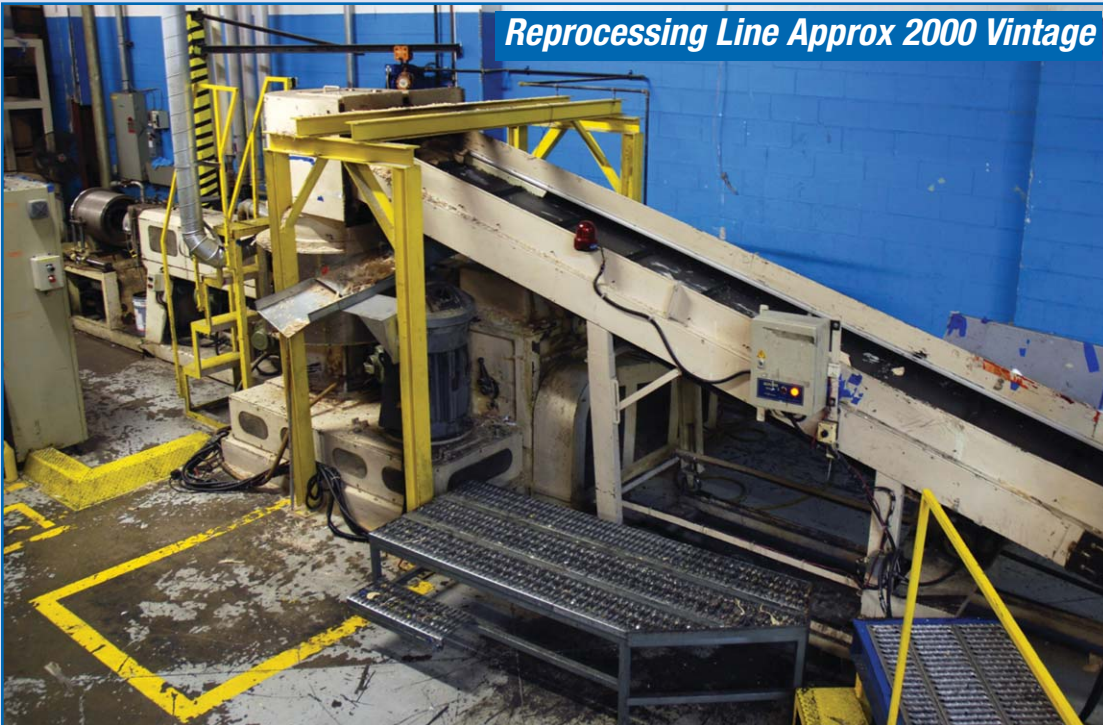
FKI 100 mm Complete Reprocessing Line, Including: Motivation 1,000 lb Gaylord Tilter, Infeed Conveyor, Metal Detector, 100 HP Compactor, 125 HP Extruder, 115" Barrel, 28:1, Vent, Hydraulic 150 mm Screen Changer, Water Ring Pelletizer, Shaker Classifier, Cyclone & Blower
