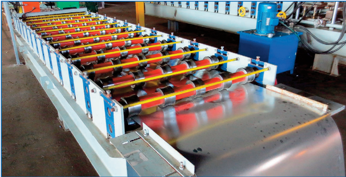
CSC ROLL FORMER/ROOF PROFILER WITH 13 STANDS, 37" WIDTH S/N 04161981 (UNIT 2)
