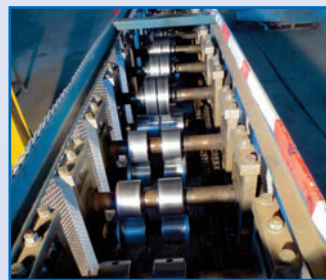
KNUDSON KS-246 ROLLFORMER/FRAMEMAKER (STUD FORMER) 10 STAND, TOOLED FOR 3.5" METAL STUDS, 2" ARBOR WITH MANUAL UNCOILER AND CUT OFF S/N 8753 (UNIT 7)
