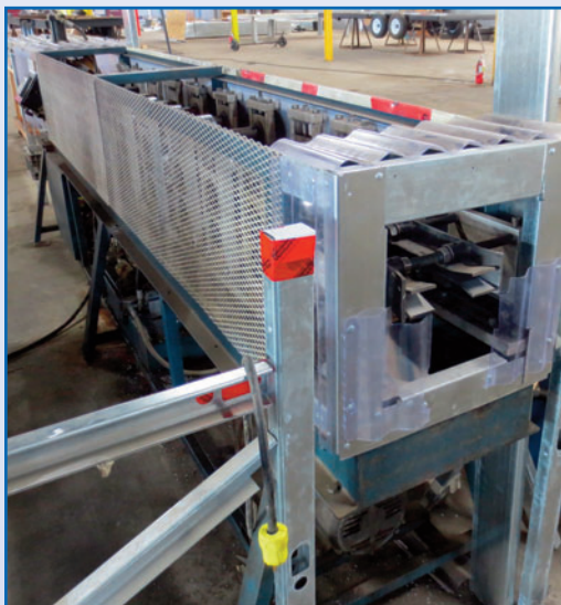
CSC ROLL FORMER/ROOF PROFILER WITH 13 STANDS, 37" WIDTH S/N 04161981 (UNIT 2)
