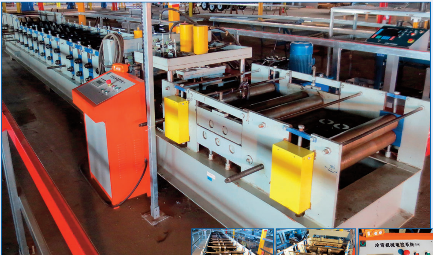
KNUDSON KS-310SF ROLL FORMER/FRAEMAKER WITH CYGK CONTROL, 3 STAND ENTRY ROLLS, 4 STAND EXIT ROLLS, 10 ROLLS (MAIN FORMING SECTION), ADJUSTABLE CHROME TOOLING, UNCOILER, CUT-OFF S/N 10275 (UNIT 4)
