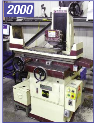
CHEVALIER 6" X 18", Model FSG 618M Hyd. Surface Grinder
