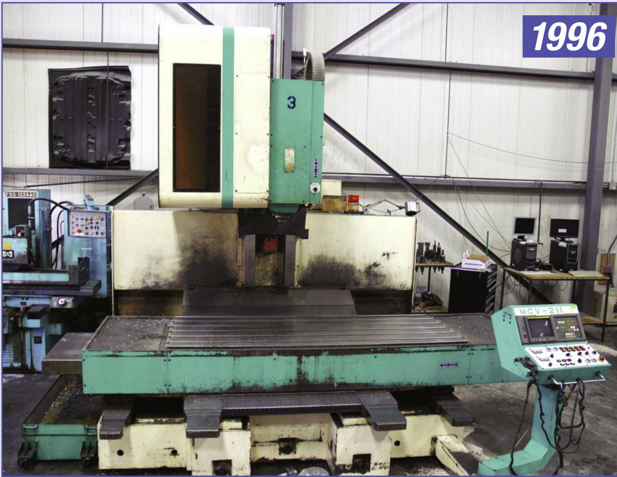
DAHLI Model DL MCV2100 CNC Vertical Machining Center
