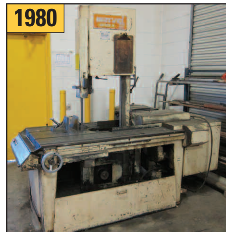
Marvel Series 8 Mark I Tilting Frame Vertical Band Saw, 18" x 20" capacity, clamping, s/n 821887-W, New 1980
