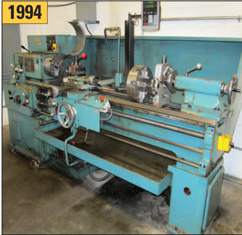
16" x 60" TOS SN-40C Engine Lathe, 8.7" swing OCS, 2000 RPM, 7.8 HP, Taper, DRO, I/M threading, s/n 08401597, New 1994
