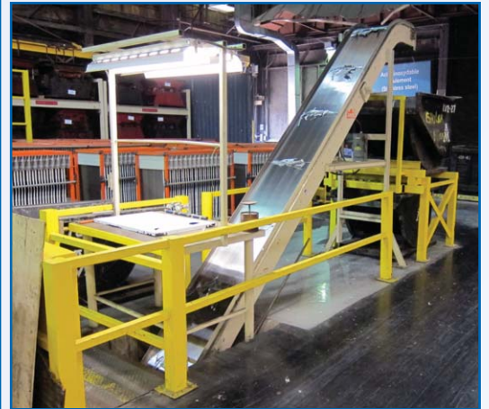
ERIEZ 250' MAGNETIC SLUG CONVEYOR SYSTEM
