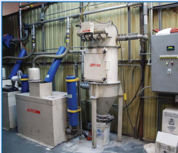
MOULDTEK 40 HP VACUUM LOADER & DISTRIBUTION SYSTEM
