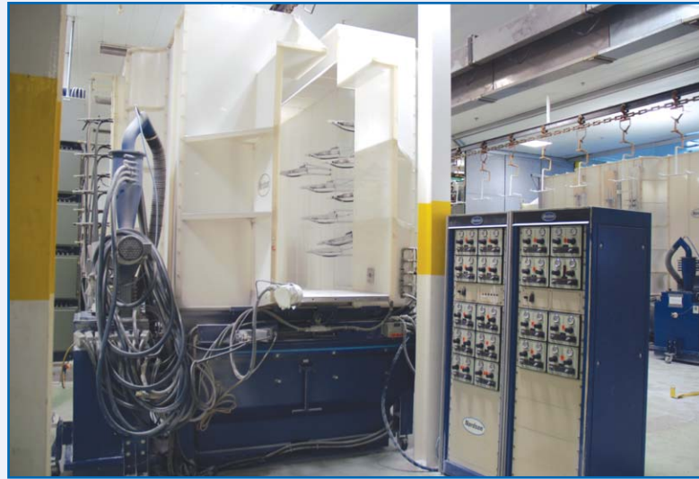
NORDSON HORIZON 4004 ELECTROSTATIC POWDER COAT PAINT BOOTH SYSTEM
