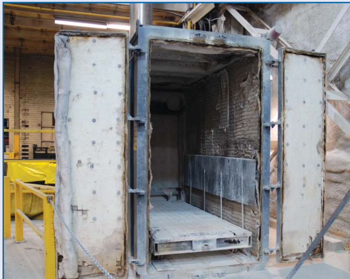
CONTROLLED PYROLYSIS PRC412 4722 DBL DOOR BURN-OFF OVEN
