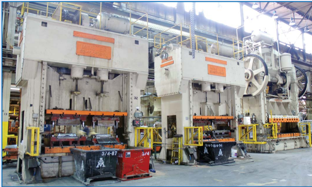
VIEW OF 2 MINSTER 400 TON & HAMILTON 1,000 TON STRAIGHT SIDE PRESSES
