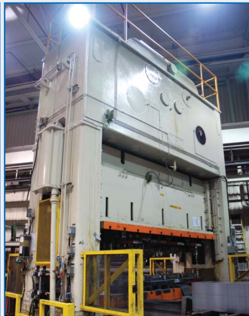
VERSON S2-300-144 STRAIGHT SIDE DBL CRANK PRESS
