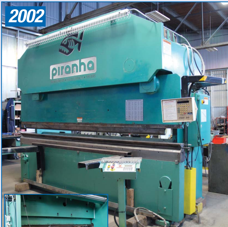
PIRANHA Model 25012, 250 Ton X 12ft CNC Hyd. Press Brake With 8" Variable Stroke, 17" Open Height, 90 IPM Approach Speed 20hp, 10'6" Between Housing, 8" Throat, Full Function Pedestal Control With Dual Palm Buttons, Automec CNC 99 2 Axis Cnc Back Gauge, (2) 36" Support Arms, 12ft 4 Way Die And Various Press Brake Dies, 37 000 Lbs, S/N 1011
