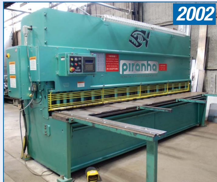
PIRANHA Model TC3/8-12, 3/8" x 12ft Hydraulic Shear With CNC Full Programmable Back Gaugefront, 24 SPM, 15 Holddowns, 20 HP, 24 500 Lbs, 49" Squaring Arm, (3) 24" Support Arms, S/N T3/8-12-1002
