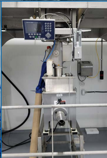
IMCS HYDRAULIC BIN DUMPER W/ HOPPER, CONVEYOR, FEEDER, WEIGHING TERMINAL, ETC.
