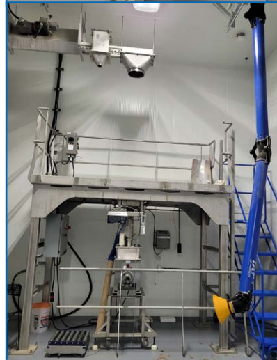
IMCS HYDRAULIC BIN DUMPER W/ HOPPER, CONVEYOR, FEEDER, WEIGHING TERMINAL, ETC.
