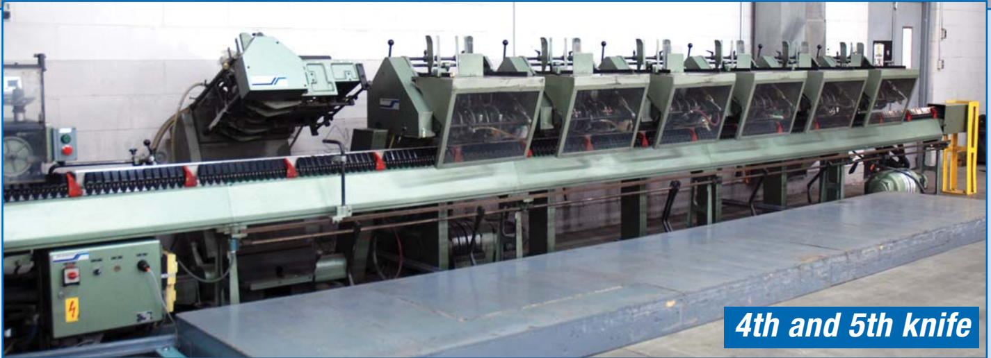
MULLER MARTINI MODEL 225 BINDER SN 942003B378 WITH 6 FEEDERS, 1 COVER FEEDER, 4 STITCHING HEADS
