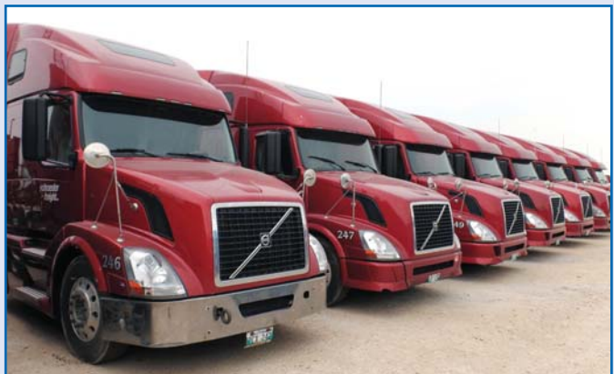
(9) 2012 VOLVO VNL64T670 T/A SLEEPER TRUCK TRACTORS C/W DD13, 425hp, Autoshift, Air Ride Suspension, 12,350 lb fronts, 40,000 lb rears, 220 in. WB, 60 in. sleeper, Espar heater, 11R22.5 Rubber
