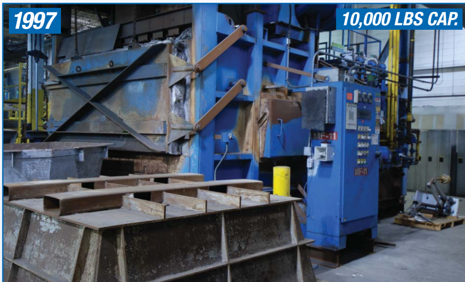
LINDBERG/MPH REVERBERATORY MELTING FURNACE
