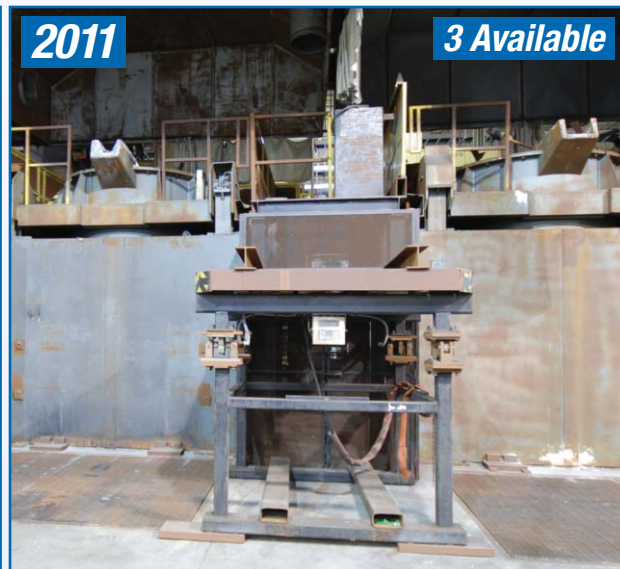
AJAX/TOCCO PACER II CORELESS INDUCTION MELTING FURNACE
