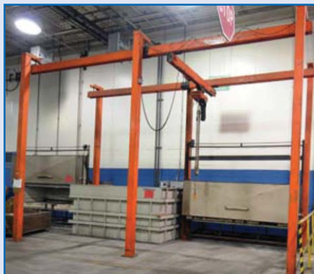
GORBEL FREE STANDING FLOOR SUPPORTED CRANE SYSTEM
