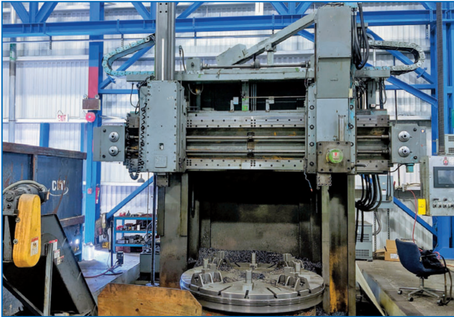
PIETRO CARNAGHI VERTICAL TURRET LATHE, 70" 4-JAW CHUCK, TWIN HEAD, CNC TOUCH SCREEN CONTROL, TITAN CHIP CONVEYOR, HYDRAULIC POWER PACK, ELECTRICAL PANELS, ETC.
