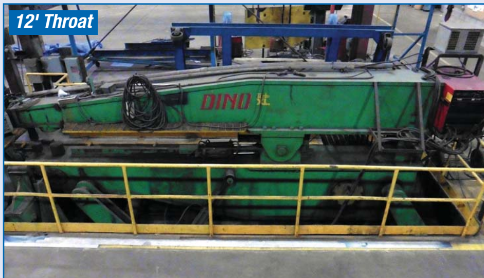
DINO Turbo XL Hydraulic Inside Seam Fitting & Welding Machine
