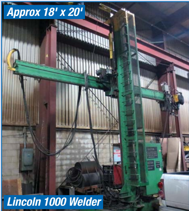
CAMTRON Welding Manipulator
