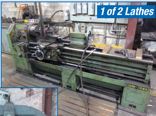
VICTOR 18" x 75" Engine Lathe, Model 2080
