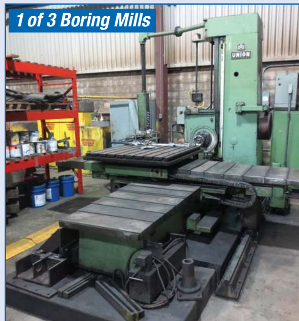
UNION 4" Horizontal Boring Mill, Model BFT-102
