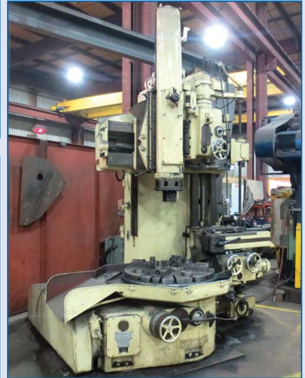
BERTHIEZ IR9320/3 Vertical Boring Mill
