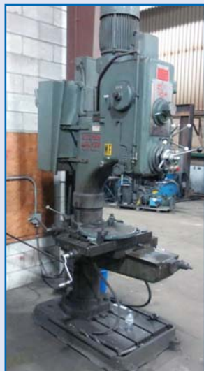
KITCHEN WALKER V2 Gear Head Drill Press
