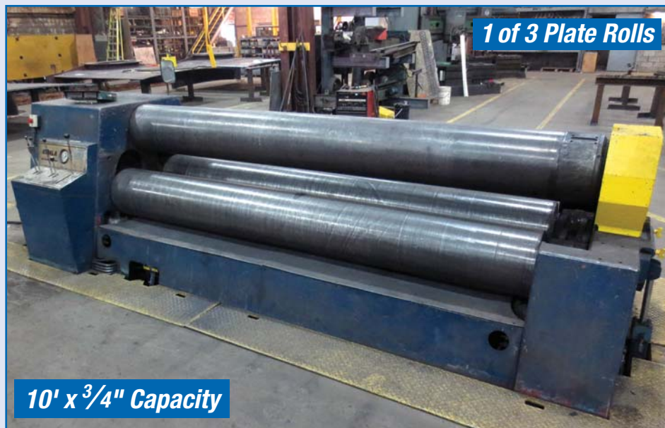
PULLMAX PV7H Hydraulic Pyramid Rolls, 10' x 3/4"
