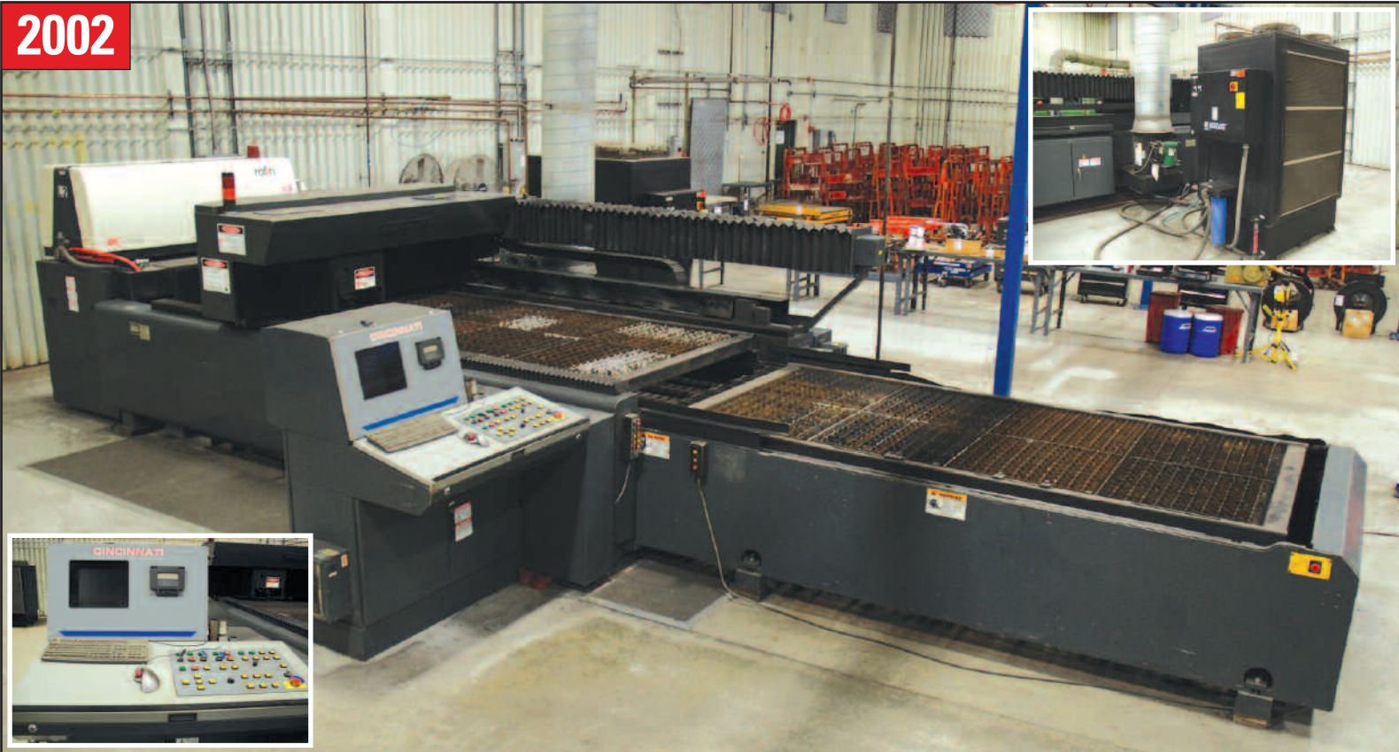
2002 CINCINNATI 3,500 WATT 5' X 10' LASER CUTTING TABLE MODEL CL-7A, WITH SHUTTLE
