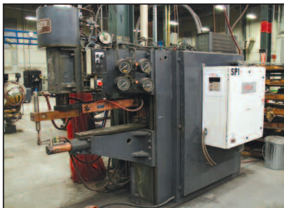
SCIAYKY 150 KVA SPOT WELDER TYPE RM00.3STO-150-36
