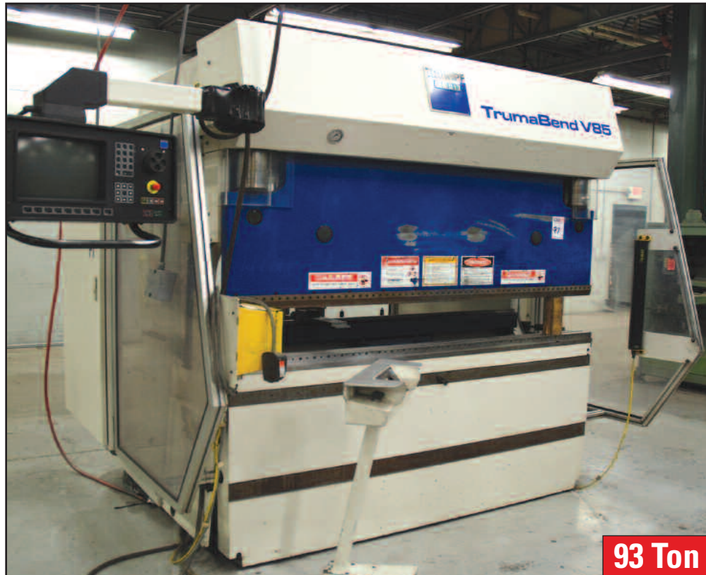
TRUMPF TRUMABEND 6.5' (80") X 93TON, MODEL V85
