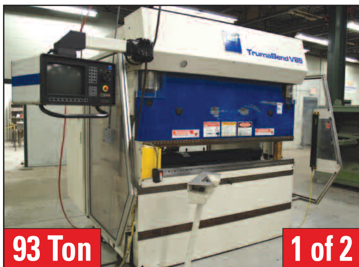
TRUMPF TRUMABEND 6.5' (80") X 93TON PRESS BRAKE MODEL V85
