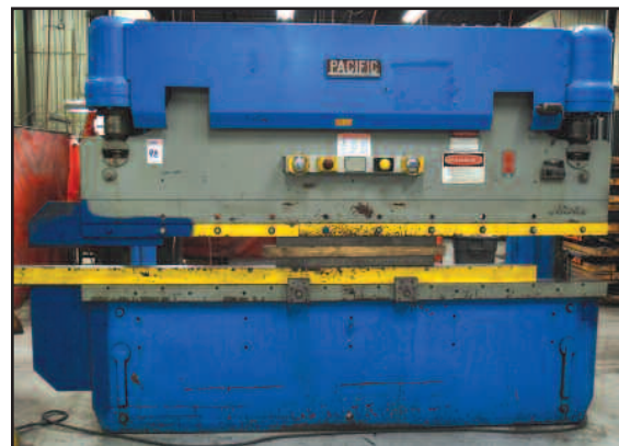
PACIFIC 10' X 90TON (10 GAUGE) MODEL J SERIES J90-10
