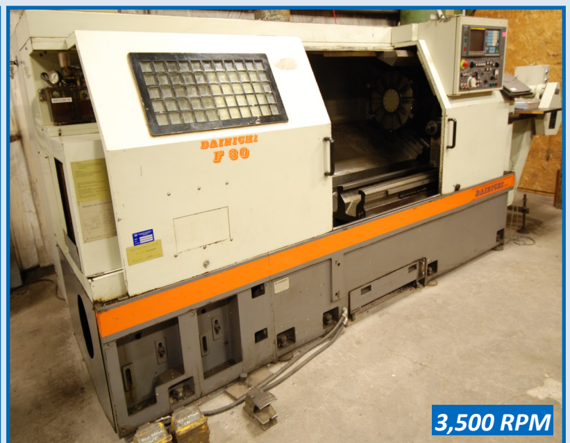
DAINICHI F30 CNC LATHE, FANUC SERIES O-T CONTROL, 12" 3-JAW CHUCK, 21.7" SWING OVER BED, 13.8" MAX MACHINING DIAMETER, 50" BETWEEN CENTERS, 3,500 RPM, 12-STATION TURRET, TAILSTOCK, S/N 23484
