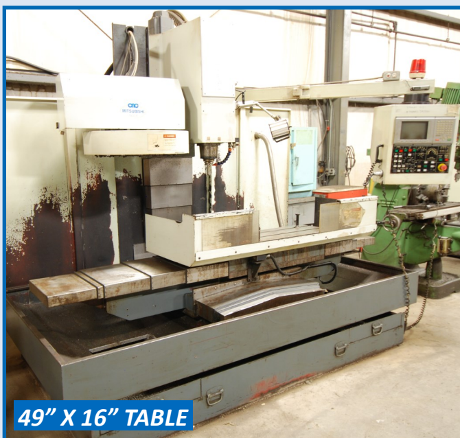
MITSUBISHI VMC-405 CNC VERTICAL MACHINING CENTER, MITSUBISHI CONTROL, 49" X 16" TABLE, 16 ATC, TRAVELS: X-39.58", Y-18.89", S/N C405-101
