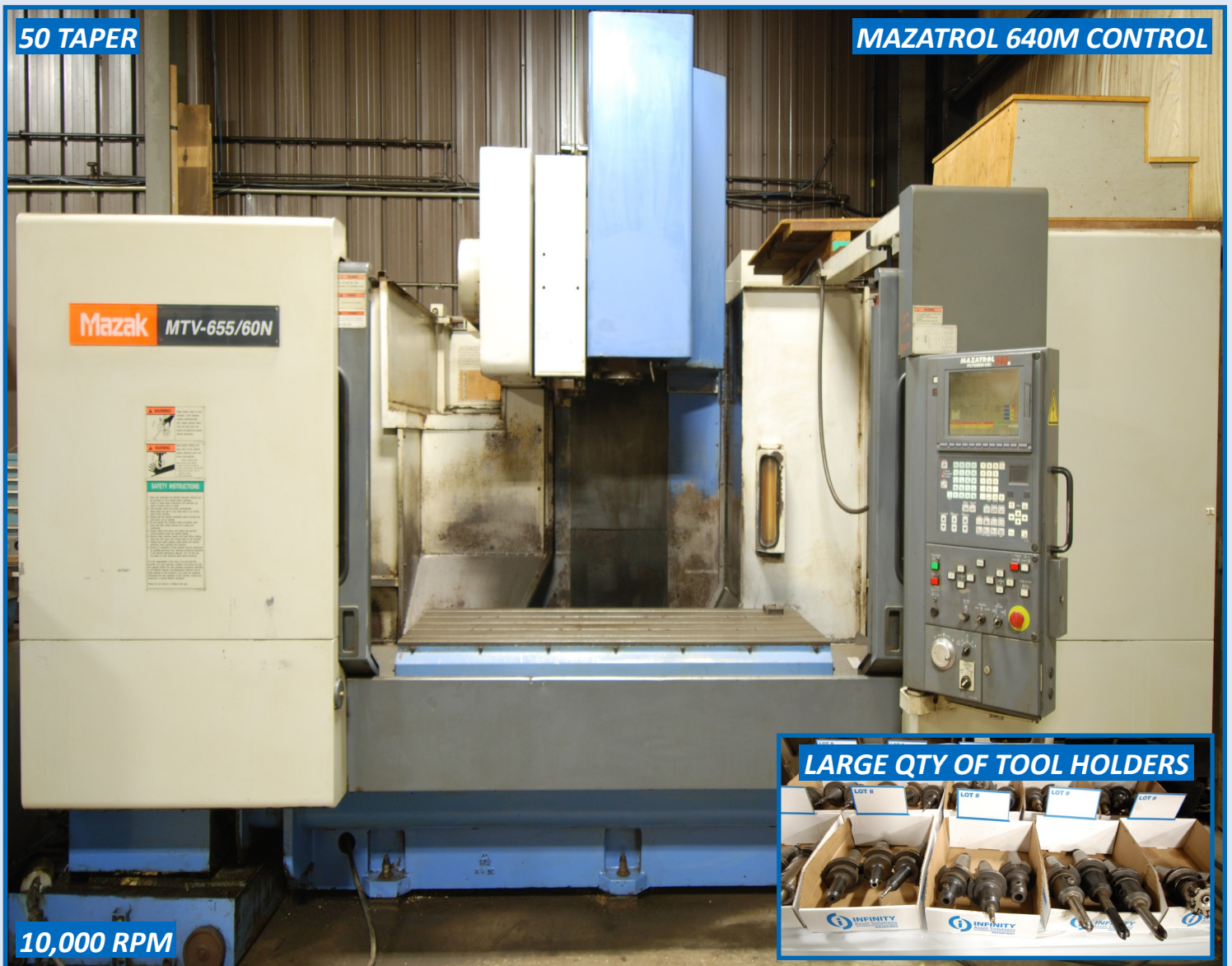
MAZAK MTV-655/60N CNC VERTICAL MACHINING CENTER, MAZATROL 640M PC-FUSION-CNC CONTROL, 64" X 26" TABLE, 10,000 RPM, 25HP SPINDLE, 30 ATC, TRAVELS: X-59.05", Y-25.59", Z-25.59", 50 TAPER, S/N 138408, JORGENSON CHIP CONVEYOR
